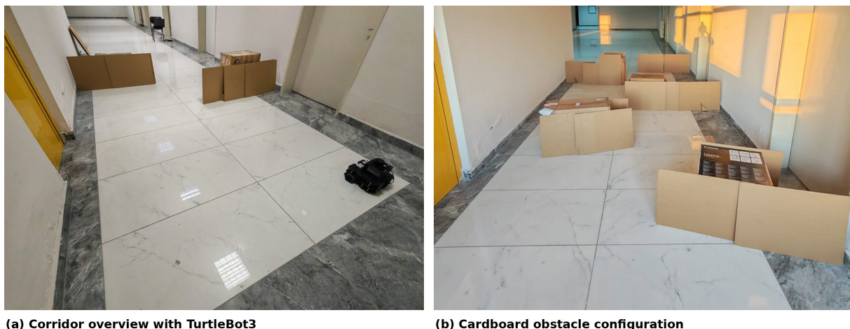
Figure 11. Physical evaluation corridor, 3.3 × 7.6 m. (a) Corridor overview with the TurtleBot3 Waffle Pi at the start mark. (b) Cardboard obstacle configuration. The Scenario 2 and Scenario 3 layouts are specified in Section 7.2. Obstacles are cardboard throughout; no human participants took part in any trial.
