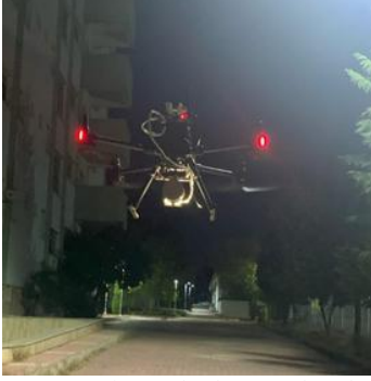
Fig. 1. The complete 3D mapping payload mounted on the DJI Matrice M350 RTK UAV
