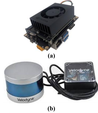
Fig. 2. Main payload components: (a) the NVIDIA Jetson Orin NX; (b) VLP16 Lidar sensor.
